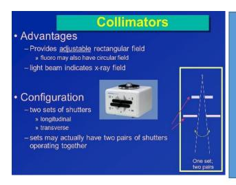
Collimator is the best all round X-ray beam restrictor ,These are two types:
