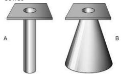
Cones are usually flare shaped, Ideal geometric configuration for an X-ray beam restrictor.
